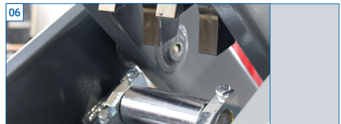
The cylinder raising support with step lever and rollers conducts a pure rolling movement. No sliding movement between the moving parts, meaning it is low noise, wear resistant and nearly maintenance-free.
