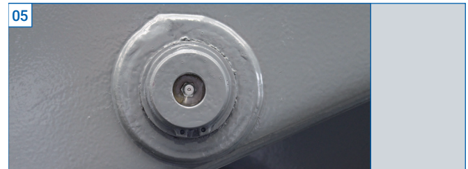
Scissors main bearing with Teflon bearing bushing and lubrication nipple, long service life and emergency running qualities.
