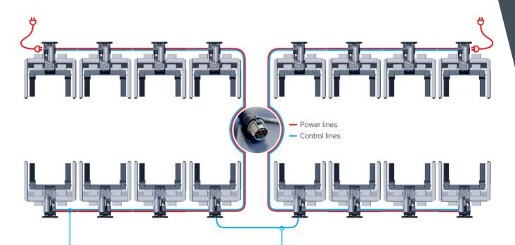
Unique double security. If the radio connection is interrupted, the charging cable can be used for data transmission to guarantee constant operation.
