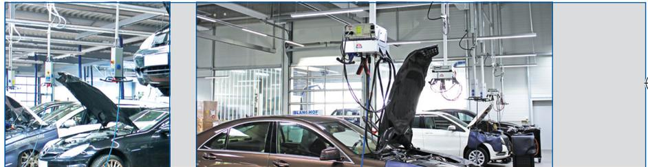
Installation examples of MAHA media supply during workshop operation. The E-BOX versions are individually adjustable to each workstation and ensure ergonomic working.
