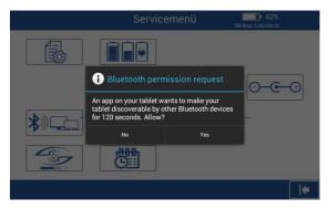
Confirm the request with 'Yes'. The headlight tester is now discoverable by other Bluetooth devices for 120 seconds.
