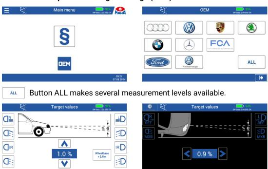
Use the Down button to navigate through the measurement levels.
