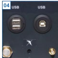
Connections for PC via USB, printer and optional Bluetooth antenna at the rear.
