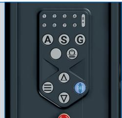
Depending on the load, high lifting and lowering speeds can be selected via separate, additional button.
