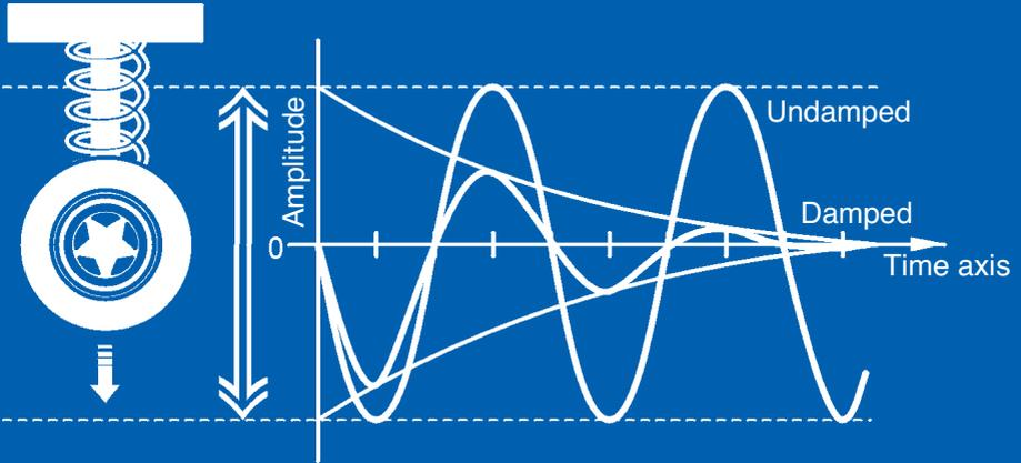
The subsiding of the oscillation amplitude (= Amplitude, oscillation amplitude) acts on the shock absorption; it brakes the oscillating wheel movements in both directions. For this, counter (damping) forces are created which
