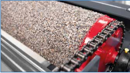
Roller surface plastic/granulate coated
