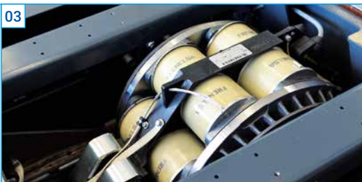
Eddy current brake for performance measurement and load simulation: 7000 N max. tractive force per axle with 1 brake Max. expansion stage with 4 brakes per dynamometer Boost function incl. temperature monitoring of the brake especially for performance measurements on electric vehicles
