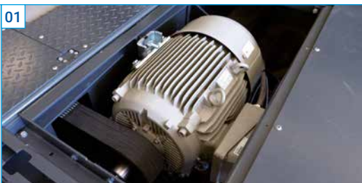
Electric machine for four-wheel synchronisation: Tracking acceleration of the non-driven axle 30 kW, 1.5 m/s 2 up to 200 km/h 30 kW, 1.0 m/s 2 up to 240 km/h All drive concepts can be tested
