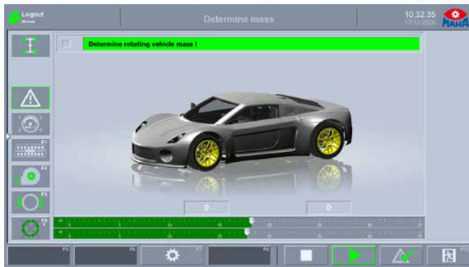
Automatic mass determination necessary for all vehicle types, as the real value per axle is unknown
